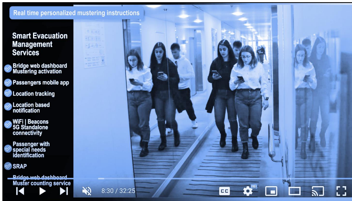
Figure 4: Technology-assisted mustering with passengers using their mobile app to be alerted and oriented towards the designated muster station
