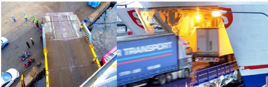
Figure 33: RO-RO Stern and Bow ramp ( www.macgregor.com )
