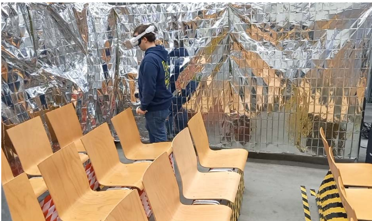
Figure 17: The MEV Mock-up was adjusted several times to allow the highest level of immersion. Seats were positioned according to the VR representation. This was a Mixed Reality Approach and allowed a real physical experience of the MEV interior.
